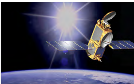
Figure 5. River surface height and slope of large rivers can be measured by radar altimetry from satellites, such as the Jason-2 OSTM shown here (image from NASA Jet Propulsion Laboratory, California Institute of Technology, https://www.jpl.nasa.gov/news/news.php?feature=6890 ).
