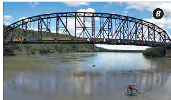
Figure 3. River surface velocities can be measured with (A) doppler radar mounted on small unmanned aerial systems as shown during field trials (B) at the Tanana River, Nenana, Alaska, July 2018.
