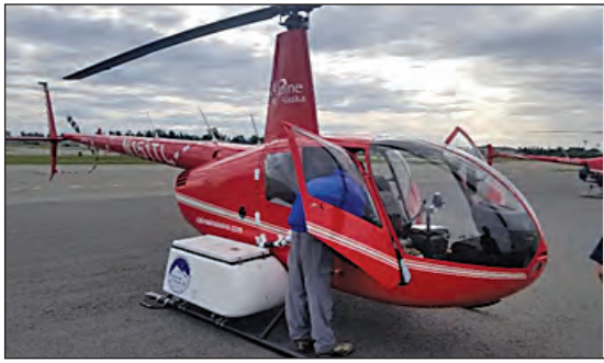
Figure 4. Measurements of river flow have been tested using a helicopter-mounted thermal camera, optical camera, and lidar; all fully integrated with a global navigation satellite system (GNSS) for direct geo-referencing, Anchorage, Alaska.
