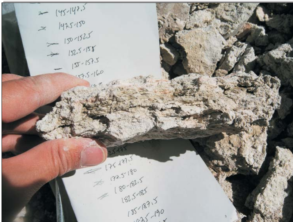
Cluster D - cemented, friable, partially lithified silt/clay, 180' - 182.5'
