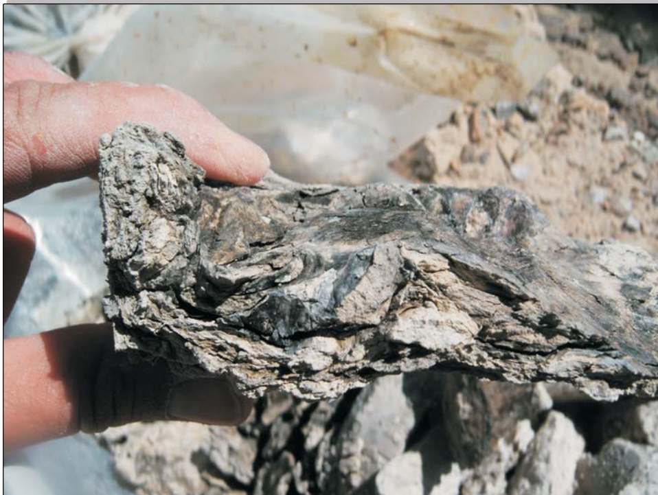
Cluster D - partially lithified, foliated clay, 192.5' - 195'
