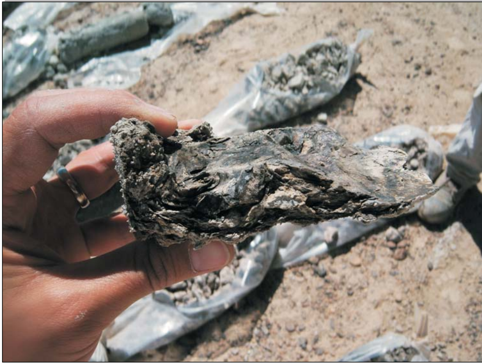
Cluster D - partially lithified, foliated clay, 185' - 187.5'
